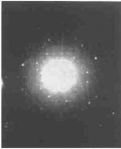
图 1 PSKNN 晶体沿 [001] 方向的背射 Laue 像 Fig. 1 Laue back-reflection photograph of a PSKNN single crystal with the beam parallel to the [001] direction
