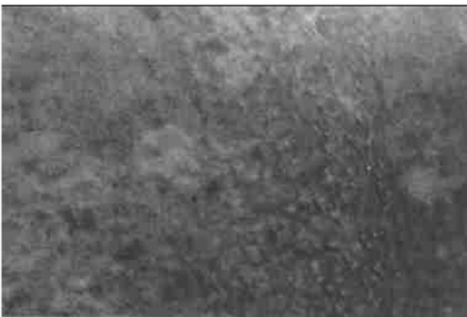
图 1 试件表面经激光气体合金化处理后的微观形貌 Fig. 1 Microstructure of the specimen treated with excimer laser (Fluence: 3.3 \text{ J/cm}^2 , \text{N}_2 atmosphere)
