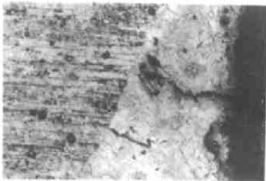
图 3 Al-Li 合金激光焊空冷焊接接头不良组织 Fig. 3 A bad microstructure of Al-Li alloy joints welded by YAG laser with air cooling
