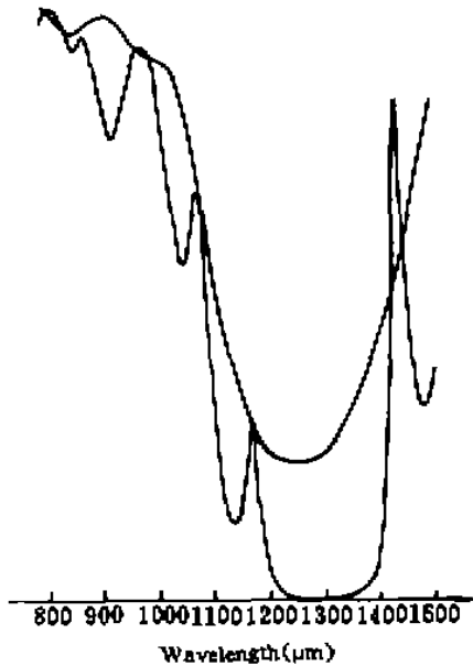
图 2 OPO 谐振腔镜的透过率曲线 Fig. 2 Transmissions of mirrors of the OPO resonator
