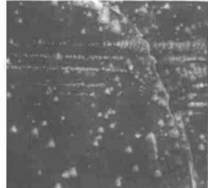
Fig. 7 Domain inversion structure formed with insufficient line-charge density
