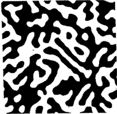
Fig. 2 Computer-simulated 2D geometry for a 23 \times 23 fan-out binary phase grating in a period. The black represents phase \pi ; The white represents phase 0
