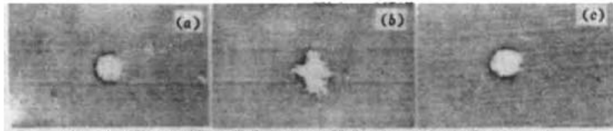
Fig. 4 The quality of the output light spots from the crystals (a) input spot; (b) Fe:LiNbO 3 ; (c) Ce:Ho:LiNbO 3
