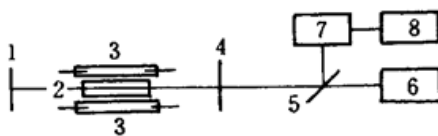
Fig. 1 Experimental setup of the flashlamp pumped Cr : LiCAF laser 1: reflective mirror; 2: Cr : LiCAF crystal; 3: Xe flashlamp; 4: output coupler; 5: beam splitter; 6: energy meter; 7: photo-diode; 8: storage oscilloscope
