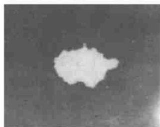
Fig. 2 Pinhole picture of a laser-produced plasma
