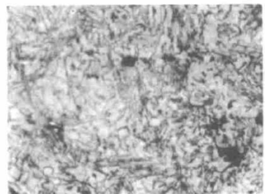
Fig. 2 Microstructure of a spray welding layer of Ni based-WC alloy on 15MnV steel ( \times 360 )
