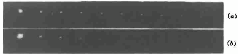
Fig. 7 The far-field beam spot bunches of the GVUR (a) and PTUR (b) lasers by wedge
