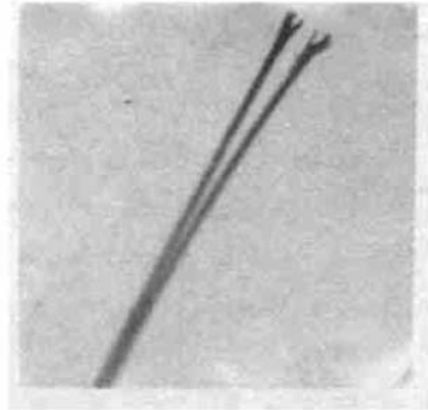
Fig. 3 The main target ( \phi 20 \mu\text{m} W wire) is cut into two pieces as the laser pulse irradiates at its tip
