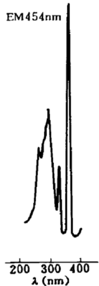
Fig. 5 Excitation spectrum of Na 5 Tm(WO 4 ) 4 crystal for Tm 3+ ion 454 nm emission at room temperature
