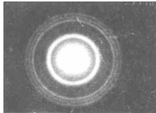
Fig. 5 Electron diffraction pattern of \alpha -CdSe sample deposited at 200 °C in a rate of 0.75 \mu\text{m}/\text{h}
