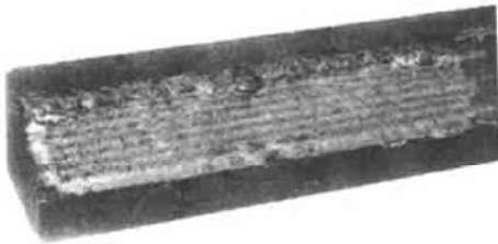
Fig. 6 Large smooth laser cladding of 6 # copper alloy on the guide block
