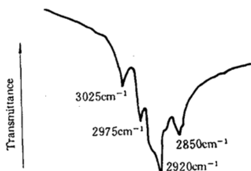
Fig. 2 IR absorption spectrum of DLC films
