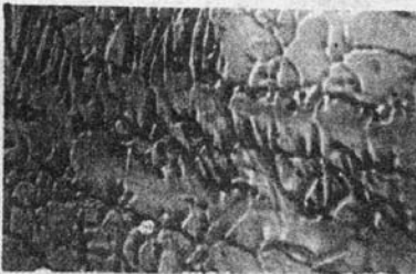
Fig. 7 Microstructure of welding bead (Amplification 1000 \times )
