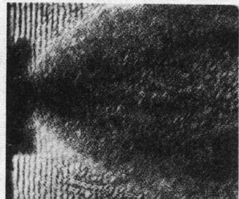
Fig. 5 Moire deflectogram of near-field structure of rocket exhausted jet by using the propellant with Al powder of 19%
