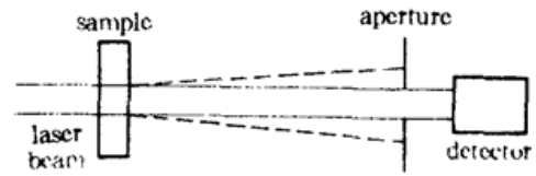
Fig. 1 Schematic diagram of optical limiter
