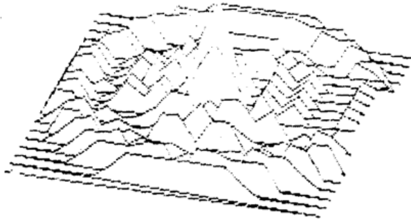
Fig. 6 Theoretical result of three-dimensional intensity distribution in the near field
