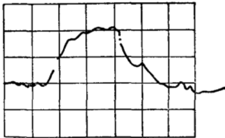
Fig. 2 Electrical pulses from the laser triggered spark gap
