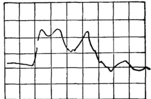
Fig. 3 Electrical pulse from the first optoelectronic switch
