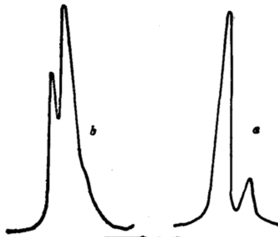
Fig. 4 Distribution of molecular weight of products obtained from Exp. (1)(a) and Exp. (3)(b)
