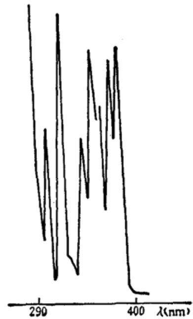
Fig. 7 Excitation spectrum of Na 5 Tb(WO 4 ) 4 crystal at room temperature
